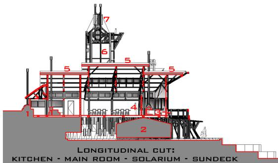
Figure 10: Main Room Section and any energy-saving features used. (Author's design) Key: 1. Wood-stove, 2. Rainwater tank (100.000 l), 3 -Stone-floor Solarium, 4. Trombe wall, 5. Roof-lawn, 6. Tower for water tank, 7. hot-air flue, viewing platform and wind turbine for water pumping.
