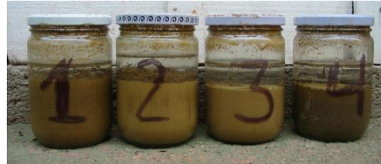
Figure 4: Soil Samples after the Sedimentation Tests. (Author's archive)
